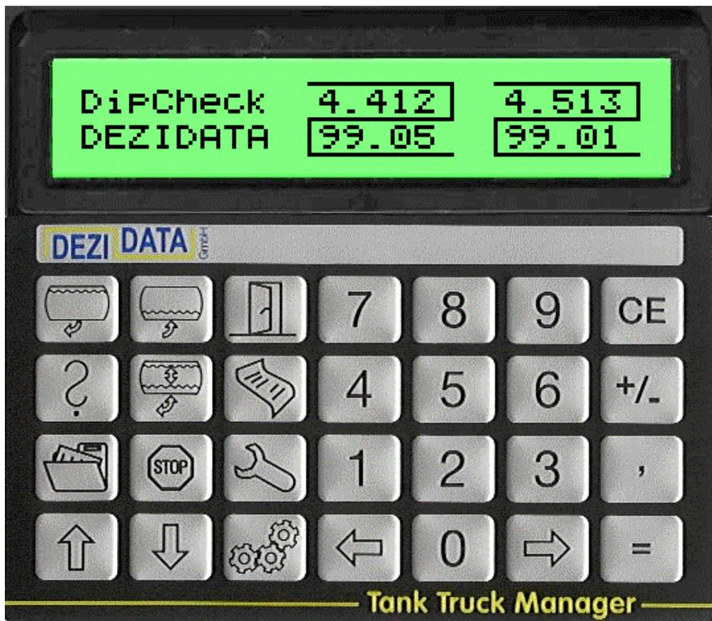
Picture 1 Keyboard and display of the TANK TRUCK MANAGER
